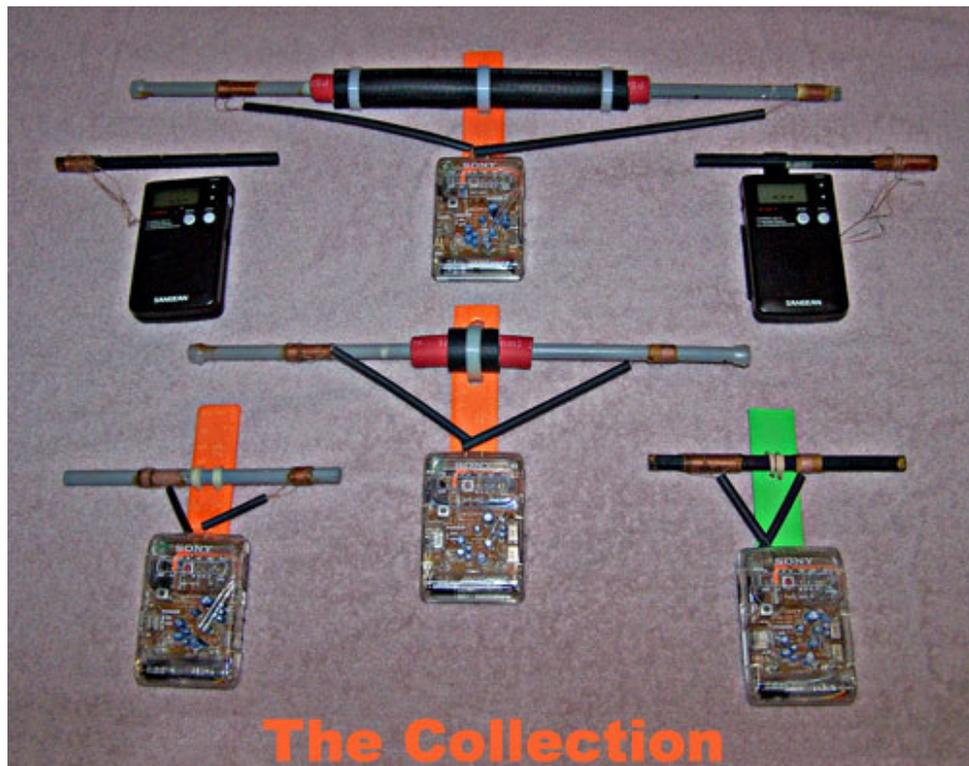
**Construction Techniques** The hobbyist has a choice of winding new coils with Litz wire on homemade movable forms, or using recycled coils on forms provided on the vintage loopsticks. All of the described models were quickly constructed by using recycled coils on
