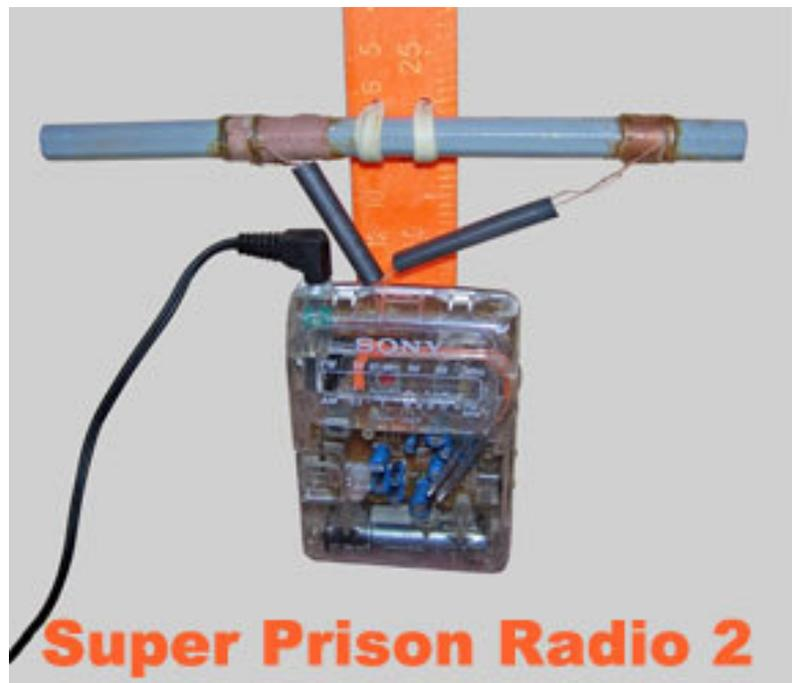
edge out the classic ICF-2010 on all frequencies (although the 2010 retained a large advantage in selectivity and spurious rejection). This “SPR2” model was constructed of both an ICF-S5 recycled 6.25” loopstick, and also a 7” antenna from the Channel Master “Super Fringe” 8-transistor model (more later, under “Construction Sources”).
