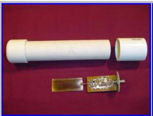
The Mini-Whip consists of a small piece of copper for the antenna and a 2-stage preamplifier. The completed antenna is enclosed in PVC pipe for weather protection.
