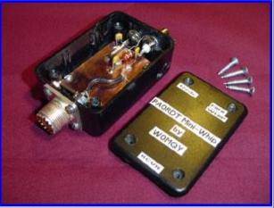
The power adapter with a BNC connector on the antenna input and a SO239 for the receiver connection.
