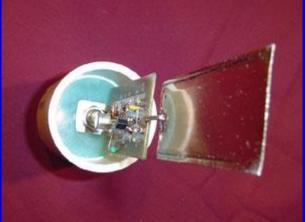
End view of the antenna. There is a BNC connector mounted on the preamplifier board.
