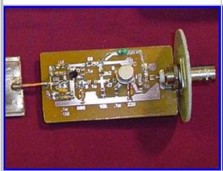
A close up of the preamplifier board. Joe used a combination of SMD and through-hole components.
