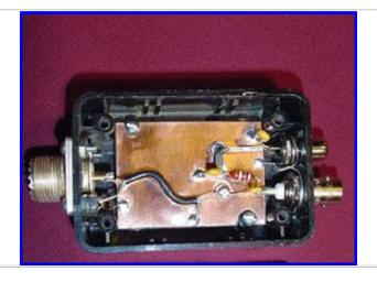
A close up of the power adapter that sends DC voltage up the coaxial cable to the antenna.
