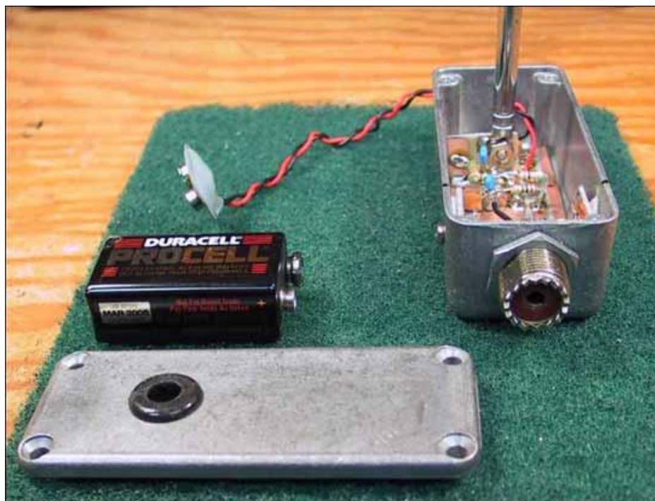
Above: The Figure 2 prototype VPA in a die-cast Hammond case. Antenna element is a 3 foot telescopic whip.
